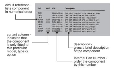
The mechanical and miscellaneous section lists the variant and common parts in IPN order.
